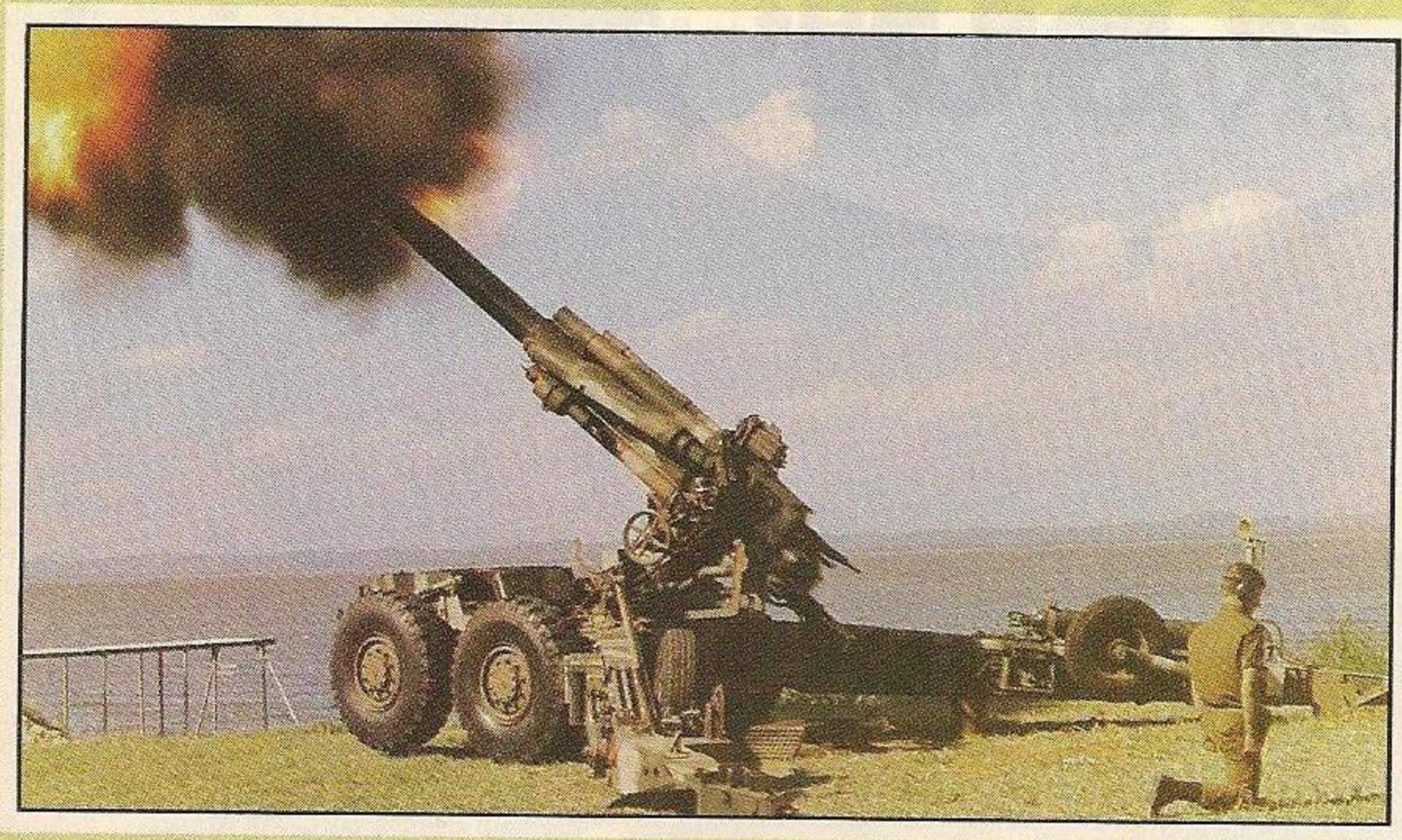
ABOVE: South African G5 155mm towed gun as used in the indirect-fire role.
