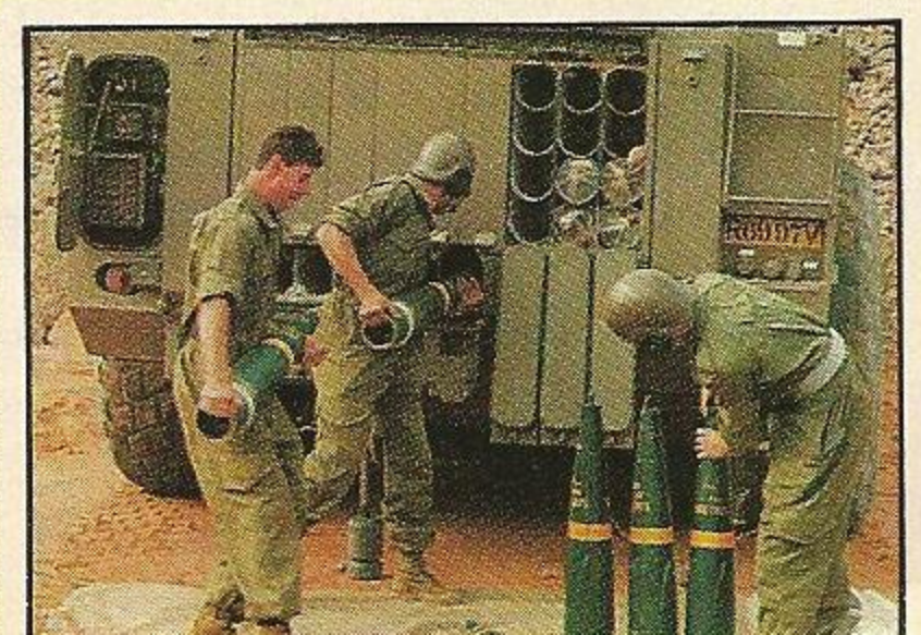
BELOW: Emergency ammunition supply for the G6 Rhino is stored in a compartment at the rear of the hull which is provided with blow-off doors.
